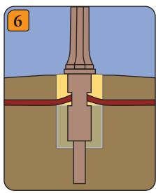
Maintain plumb while adding backfill. Tamp at 9" intervals up to bottom of cable entrances. Remove sling. Install underground cable. Make electrical connections and close handhole cover. Finish filling and tamping to 2" above final groundline.
