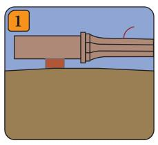
Prewire pole. Install necessary arms, luminaires, brackets, signs. Wire luminaire and handhole.
