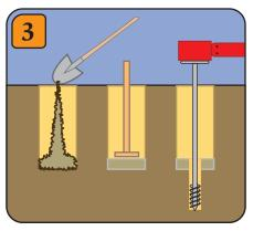
Add and tamp 6" of backfill\* to ensure correct pole setting depth and proper drainage. If pole has a stub that extends below the butt, bore a hole of that same dimension in the center of larger hole.
