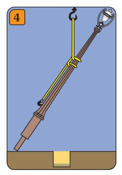
Connect hook end of a sling to pole handhole. Make two clove hitches around pole, at a point from pole top equal to one-third overall pole length. Attach sling to crane hook. Lift pole so butt end rests on ground.
