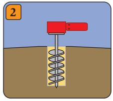
Auger a hole 10" greater in diameter than pole butt and 6" deeper than embedded length.
