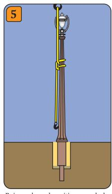
Raise pole and position over hole. Lower until butt end is resting in the center of hole bottom. Rotate pole as needed. Sight in-line from various positions with plumb bob.
