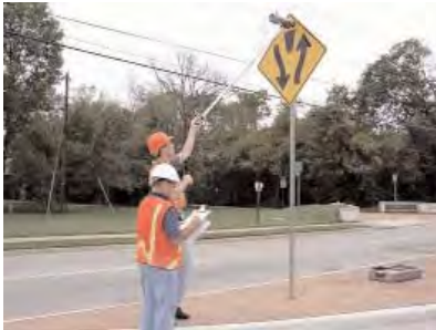
Retroreflectometers are used to measure sign retroreflectivity.
