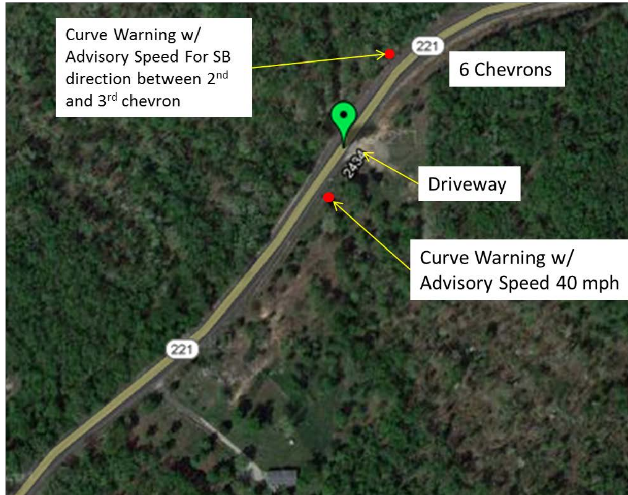
Figure 25. Photo. Missouri Highway 221 site layout.
