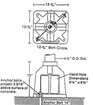
This TAPCO pedestal base is to the best of our knowledge the first designed in accordance with the 1985 AASHTO Specification for the Design and Construction Of Structural Supports for Traffic Signals, Signs, Highway Lighting, together with a wind velocity of 80 miles per hour plus gust factor.
