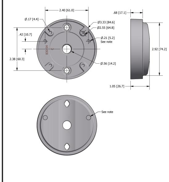
This cast aluminum Universal Bulldog Pole Mount is uniquely designed to provide either: a very strong and low profile mounting option for Polara's BullDog Push Button, or as an adapter to a variety of existing mountings. With Polara's BullDog Button attached to this mount (and directly to the pole), the main body of the button extends only 1.5" from the pole.
